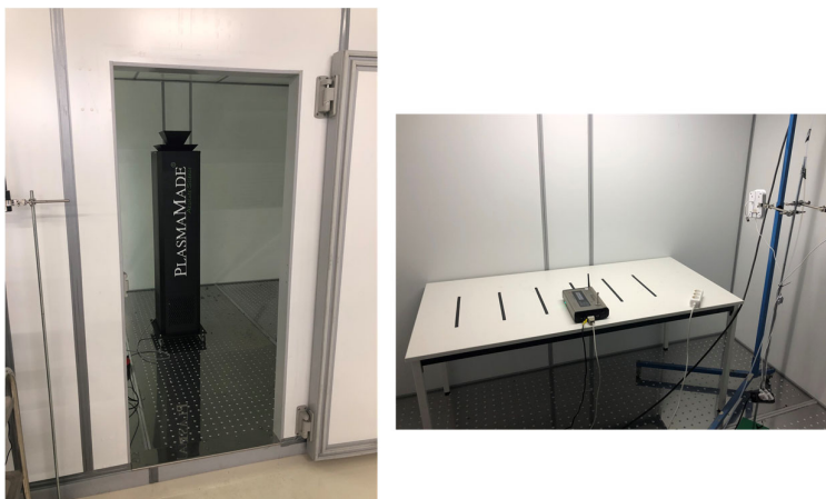
Figure 1: Left: Air cleaner in the test room. Right: Grimm 11-R particle sizer on a table in the test room.
